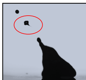
Figure 12. Puffing of a child droplet of \phi 0.5681 mm ejected from of parent droplet of \phi 2.6 mm
